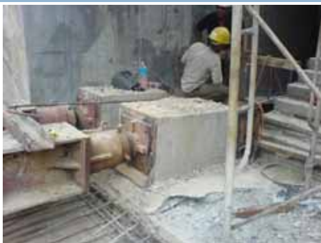
Shear Failure of Corbel Support
