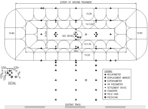
Figure 3. Instrumented layout plan.
