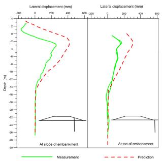
Figure 7. Measured lateral displacement of embankment.
