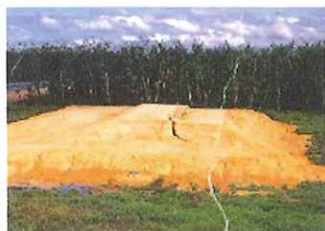
Figure 6: The Muar Test Embankment after Failure (from Malaysian Highway Authority (1989))
