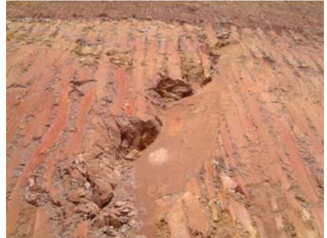
Figure 6. Daylighting joint sets observed on slope.
