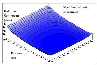
Fig. 7. Settlement profile for semi-detached house (intermediate unit).
