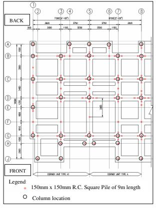
Fig. 8. Typical layout of foundation system for terrace houses.
