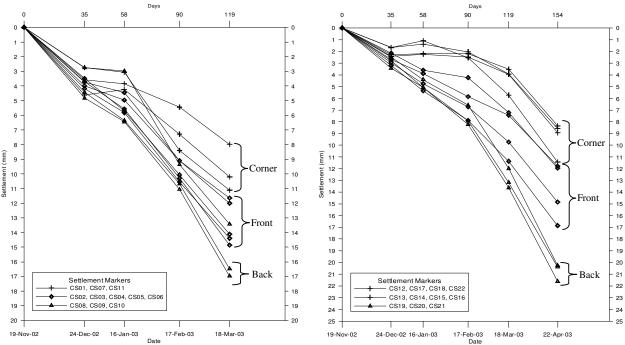
Fig. 11. Settlement monitoring results for Block 2.
