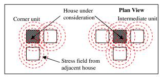
Fig. 4. Effect of adjacent houses on settlement (semi-detached house).
