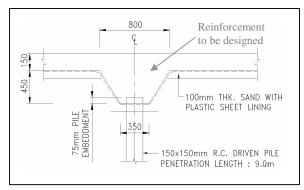
Fig. 9. Typical cross-section of strip raft foundation system.
