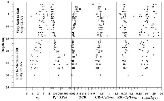
Fig. 1. Compressibility parameters for Klang Clay (from Tan et al., 2004).
