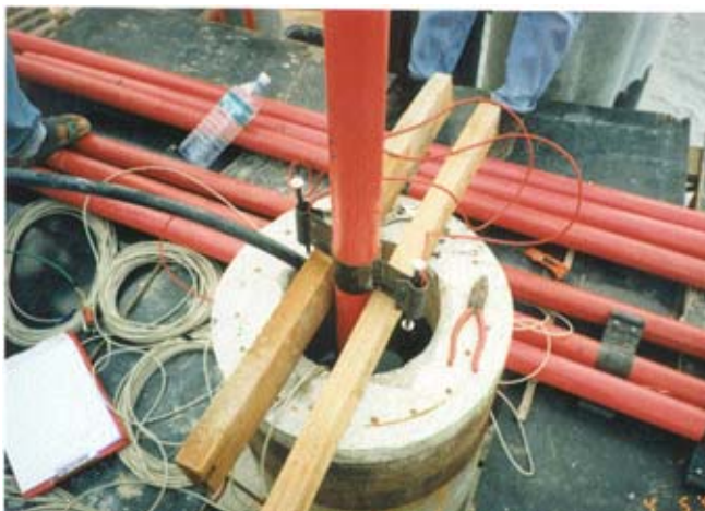
Photo 2: In the Process of Installing Strain Gauges and Inclinometer in a Spun Pile
